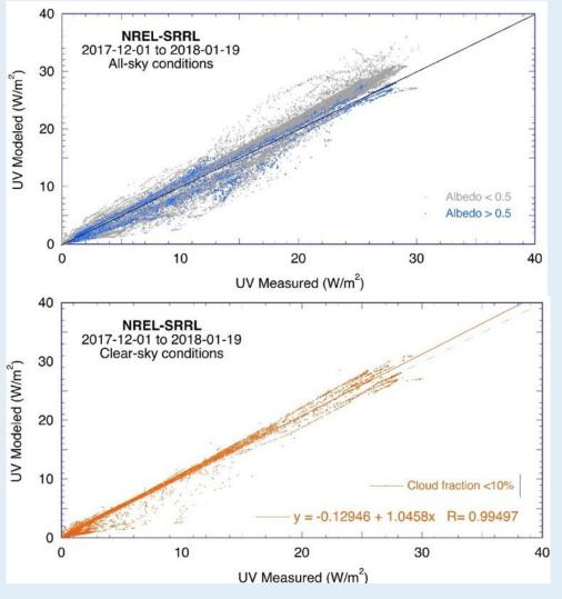
Modeled vs. measured 1-min UV global irradiance under all skv conditions at SRRL for low and high surface albedo conditions.
