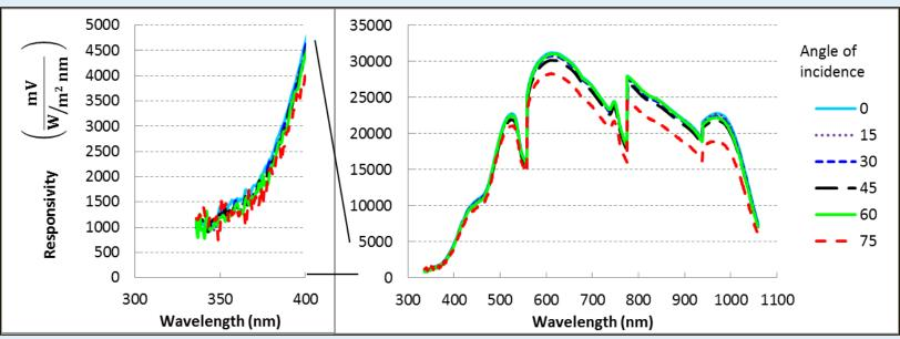
Responsivity compared to wavelength for various angles of incidence. The responsivity is nearly constant as the angle of incidence changes. Only when the angle of incidence is increased to 75° is there a noticeable change in the responsivity compared to the other angles. A detailed view of the wavelengths from 300–400 nm is shown in the left panel.
