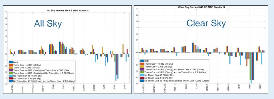
Newer radiometer designs have low cosine response and thermal offset and might not require correction.
